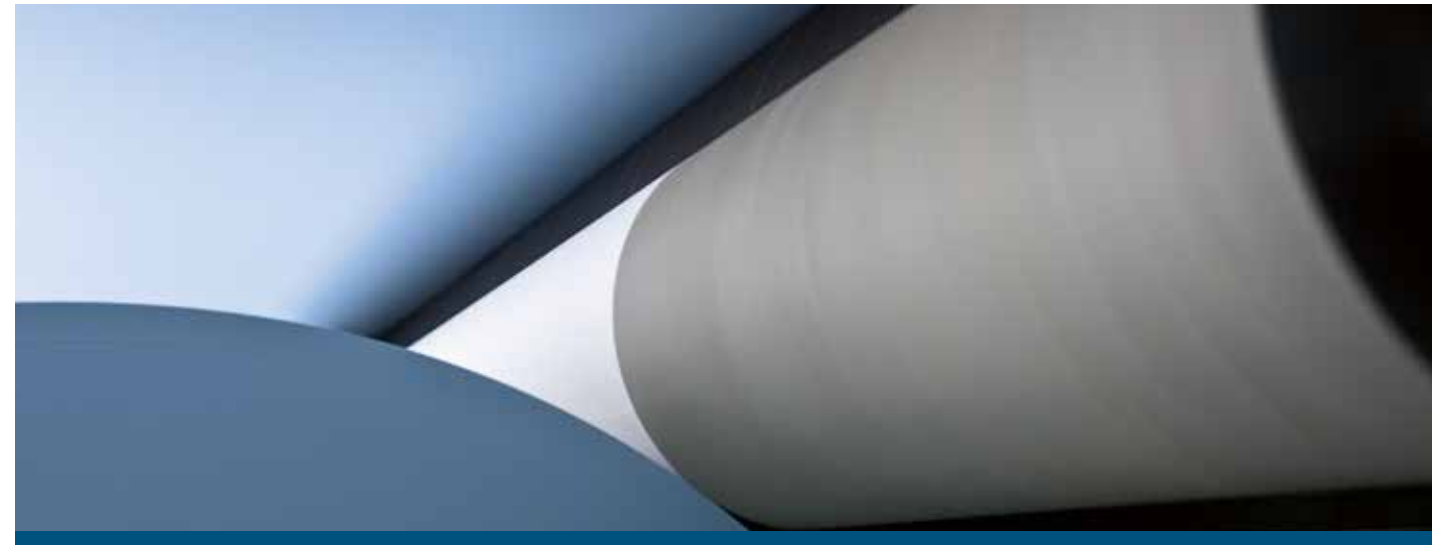
The even contact of the lay-on roller on the web reel is crucial to the winding quality.
