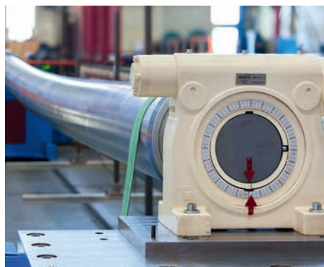
Spreader roll final test run
